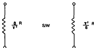
Figure 4, Load equivalent generators.
