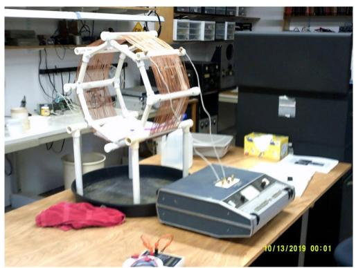
Figure 2 - PVC cage inductor.
