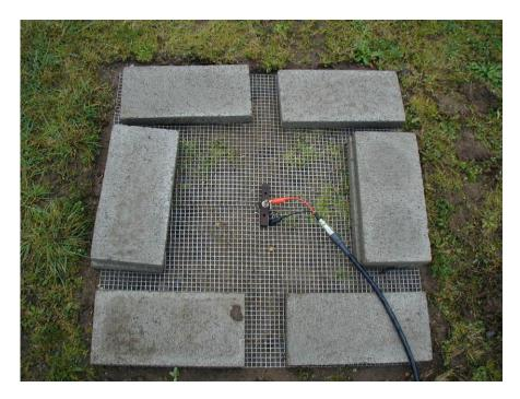
Figure 1 - Test probe and screen.
