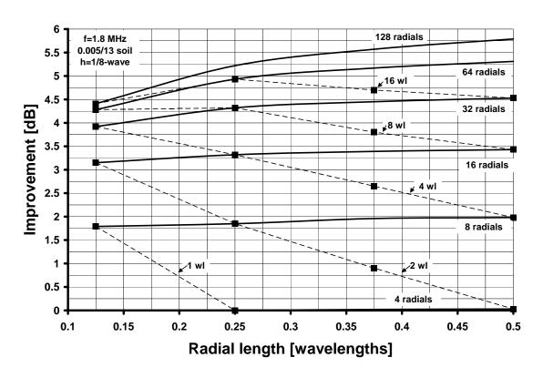
Figure 5, improvement in dB for various radial combinations for a 1/8-wave vertical.
