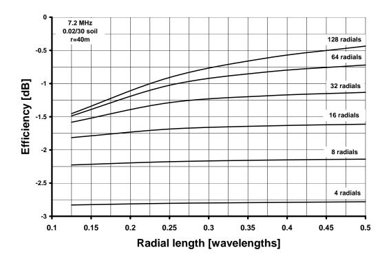
Figure 2, efficiency in dB as a function of radial number and length in very good soil. **r**=40 m.
