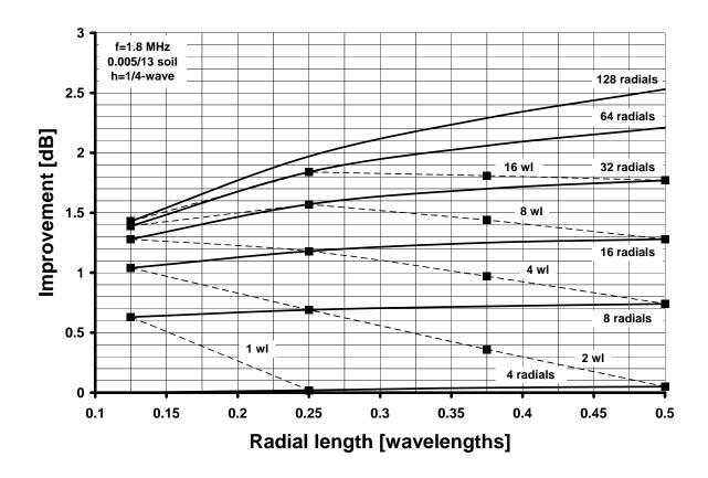
Figure 6, improvement in dB for various radial combinations for a 1/4-wave vertical.
