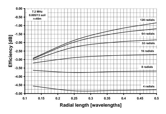
Figure 1, efficiency in dB as a function of radial number and length in average soil. **r**=40 m.
