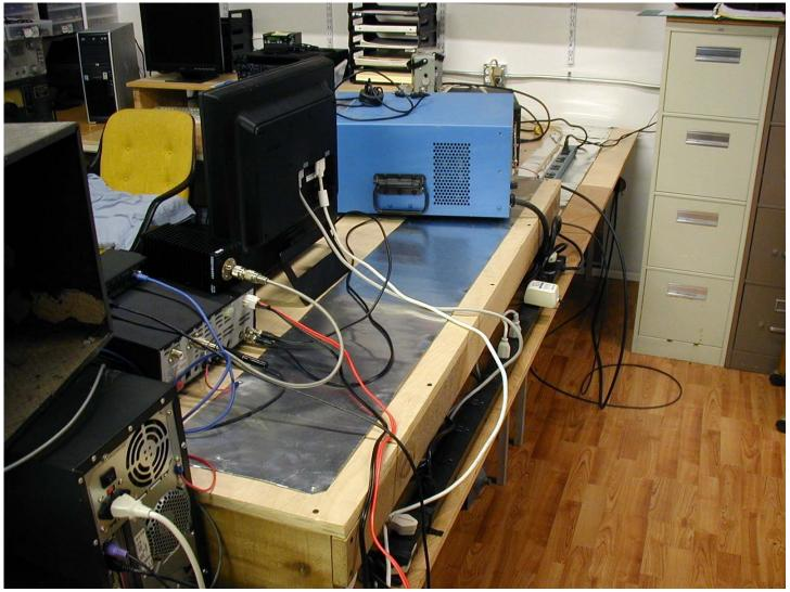
Figure 9, grounding strip inside the shack.
