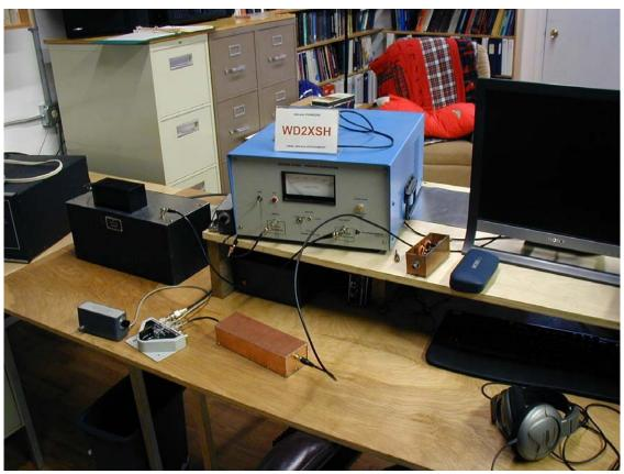
Figure 3, ENI 1040L amplifier and filters.
