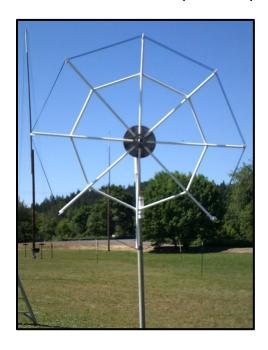
Figure 6 - Octagonal test loop.
