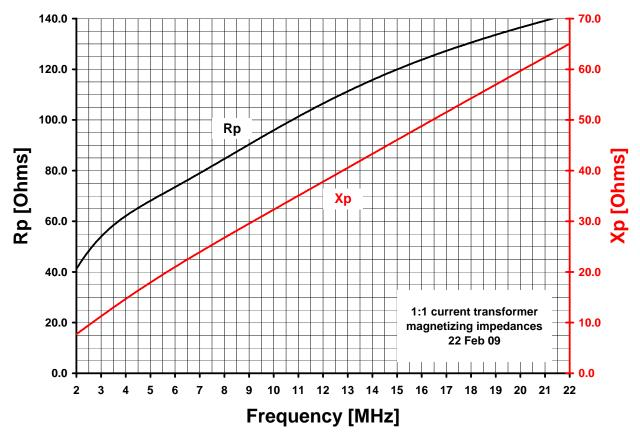
Figure 8, parallel resistance (Rp) and reactance (Xp) for the large 1:1 CT.
