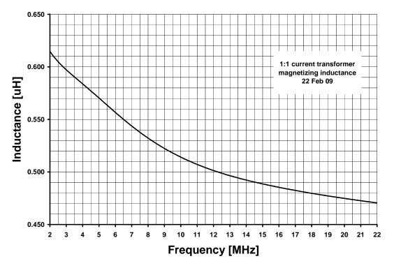
Figure 9, magnetizing inductance on the secondary.
