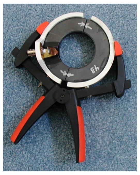
Figure 11, clamp-on current transformer.
