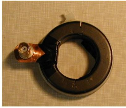
Figure 6, final assembly of the CT.
