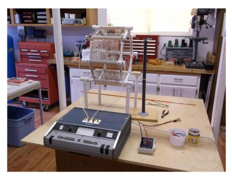
Figure 1 - Test inductor and experimental arrangement.
