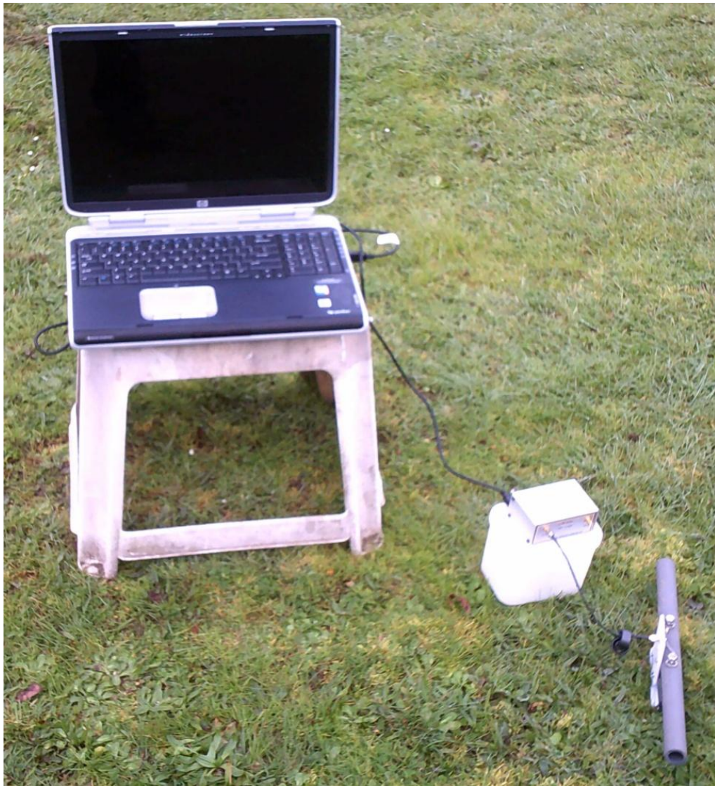
Figure 8 –VNA and laptop spaced away from ground with a choke.
