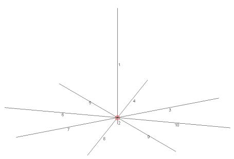
Figure 1 - typical NEC model.
