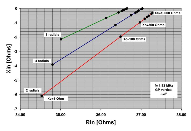
Figure 2 – Zin = Rin + j Xin for different values of choke reactance (Xc).
