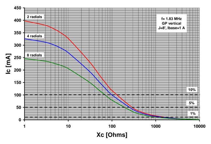
Figure 3 – choke currents(Ic) as a function of Xc.
