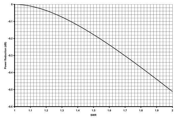
Figure 6, Power reduction due to SWR.
