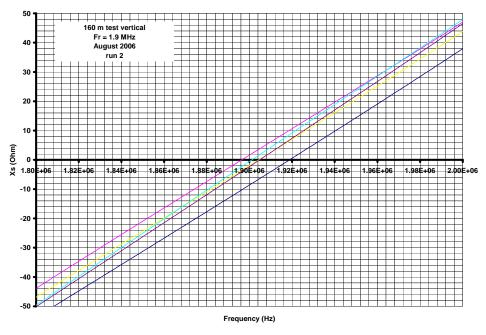
Figure 3, measured base reactance over the 160 m band.
