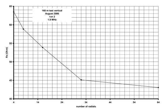
Figure 4, R<sub>s</sub> at 1.9 MHz for different numbers of radials.
