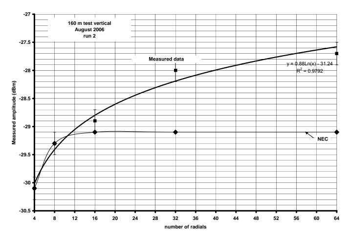
Figure 5, Measured voltage at the receive antenna as the number of radials are varied.
