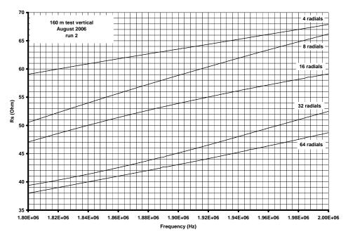
figure 2, measured base resistance over the 160 m band.
