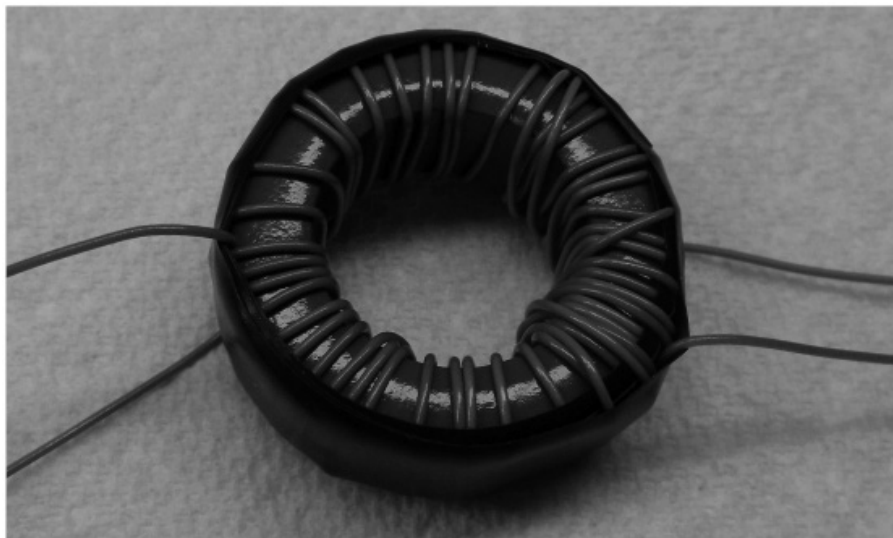
Figure 20 — Primary winding added to the impedance transformer.
