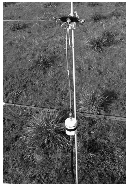
Figure 7 — Center connector and feed-point support. [Rudy Severns, N6LF, photo.]
