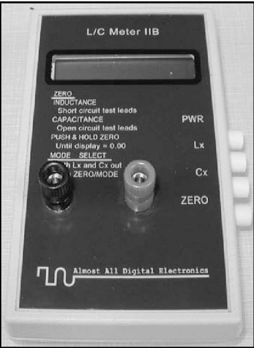
Figure A1 — I used this Almost All Digital Electronics L/C meter to measure the capacitance of the probes in air. By measuring the total capacitance of the probe and leads, and then measuring the parasitic capacitance, C p , of the part of the probe above ground along with the connecting leads, I am able to calculate the capacitance of the probe alone, C 0 .
