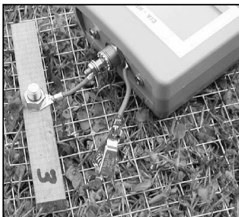
Figure 5 — This photo shows the details of how the impedance analyzer is connected to the probe and ground screen.
