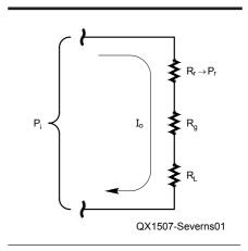
Figure 1 — This is a typical equivalent circuit for an antenna feed point resistance.
