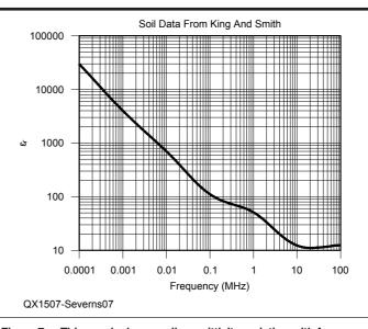
Figure 7 — This graph shows soil permittivity variation with frequency.
