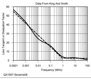
Figure 8 — Here is a graph of the loss tangent associated with the soil in Figures 6 and 7.
