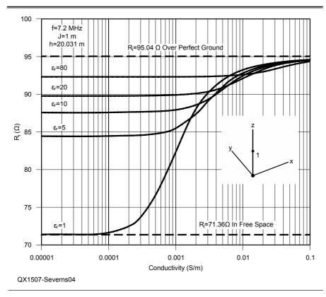
Figure 4 — Here is a graph of  $R_i$  versus ground conductivity for a ½  $\lambda$  vertical dipole at 7.2 MHz.
