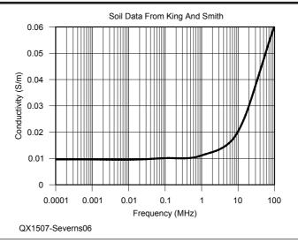
Figure 6 — This graph gives an example of how soil conductivity varies with frequency.
