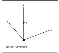
Figure 3 — This model shows a ½ λ vertical dipole, with the bottom of the antenna 1 m above ground.
