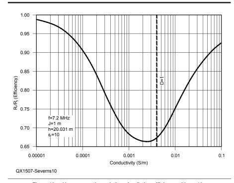
Figure 10 — Here we see the variation of radiation efficiency with  $\varepsilon_r$ = 10.
