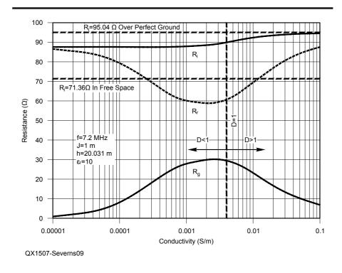
Figure 9 — Variations in  $R_i$ ,  $R_r$ , and  $R_g$  with  $\varepsilon_r$  = 10.
