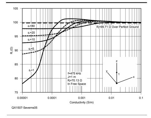
Figure 5 — This graph shows  $R_i$  versus ground conductivity for a ½  $\lambda$  vertical dipole at 475 kHz.
