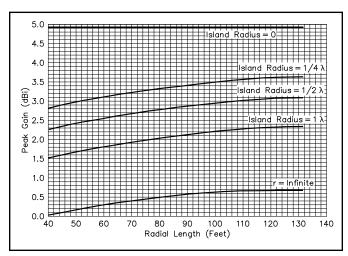
Fig 3—Peak gain for a ( $\lambda$ /4-high vertical with four, coil-loaded short radials on 160 meters, but this time where the antenna is located on a circular island in a saltwater ocean. Three different radial heights are shown over average ground. The radius of the circular island is equal to the length of the shortened radials in this model. Obviously, you should mount your antenna and radials over—or at least as close to—salt water, as you possibly can!
